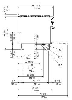
Electrical inlet (power) Gas connection
